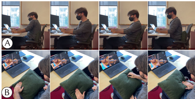
Figure 11: Tactile Sensing Pillow: Used for (A) Posture monitoring, from left to right: leaning right, leaning left, leaning back, sitting up straight and (B) Remote Control, from left to right: Play, Pause, Volume Up, Volume Down.
